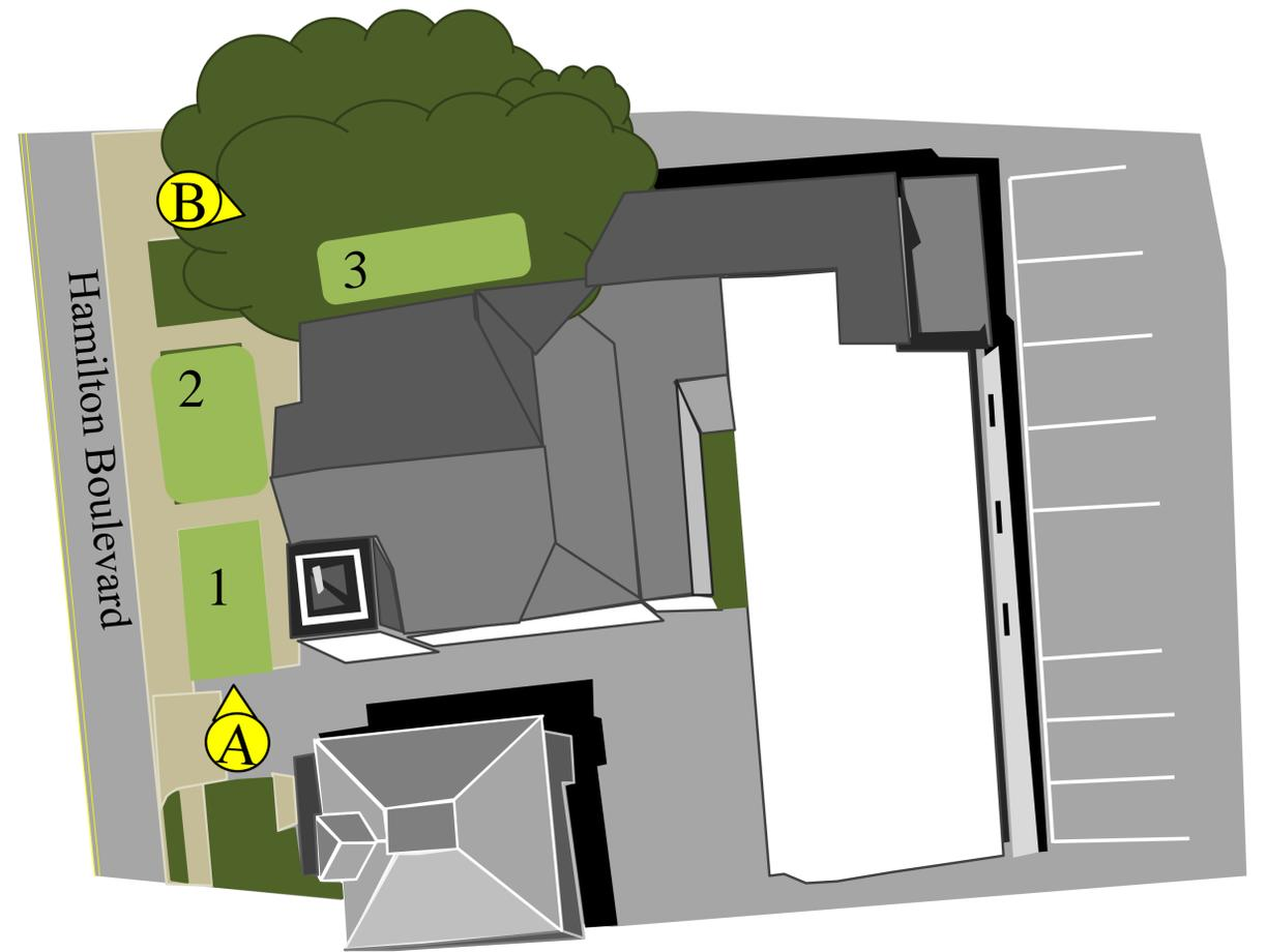
**1 BIORETENTION SYSTEMS:** Three rain gardens could be installed to capture runoff from the building's rooftop and driveway through use of various drainage methods. These rain gardens will reduce sediment and nutrient loading to the local waterway while providing beautiful landscaping to the church grounds. The gardens will also provide habitat for birds, butterflies, and pollinators.
